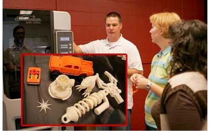
Northern's Design Drafting program has a new 3D printer. This new printer will teach our students how to design parts and build a plastic prototype of their parts so they can test their designs. This printer is the result of a Perkins grant.
